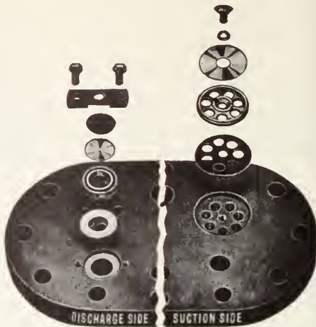
11-14. A replacement valve plate. These special valve plates are available for most refrigeration compressors. The valves and the valve seats are removable and can therefore be easily repaired. (Chicago Seal Co. Inc.)
